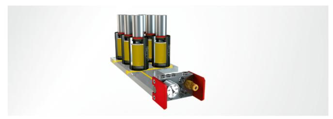
Composite plate systems consist of several nitrogen cylinders, a control panels and the composite plate. All components are connected to one another via boreholes in the composite plate. As with composite tube systems, this ensures standardised system pressure and a larger nitrogen volume, resulting in a flatter force curve.
