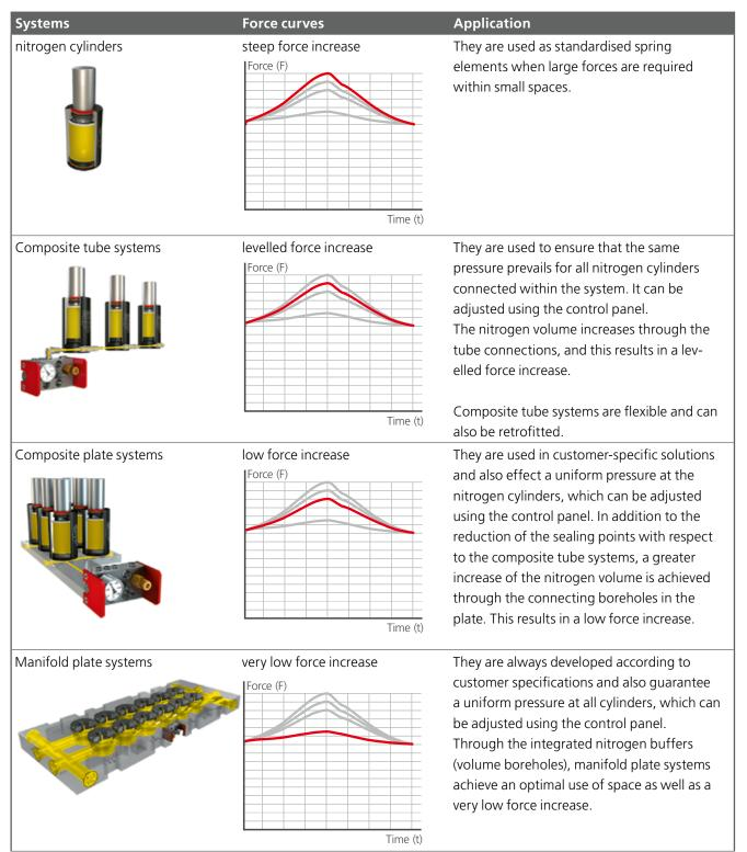
The FEM-calculated and TUV-approved design provides the highest safety standards in accordance with the PED directives (Pressure Equipment Directive). Starting at a nitrogen volume of 1 litre, pressure equipment is subject to PED directives and must also be tested and have a CE mark. Additional regulations, installation instructions etc. for our products can be found under **www.steinel.com** » Service » Operating instructions.
