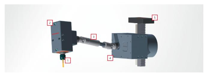
The S-Former Z is a purely mechanical solution for process-integrated tapping. The linear stroke movement of the press is converted into a rotation movement via a gear rod-sprocket pairing. This is translated in the gear to the required rotation speed and transmitted via a Cardan shaft to the tapping unit head. There, a lead screw rotates equally with the roll tap (equal pitch) and drives it into the part.
