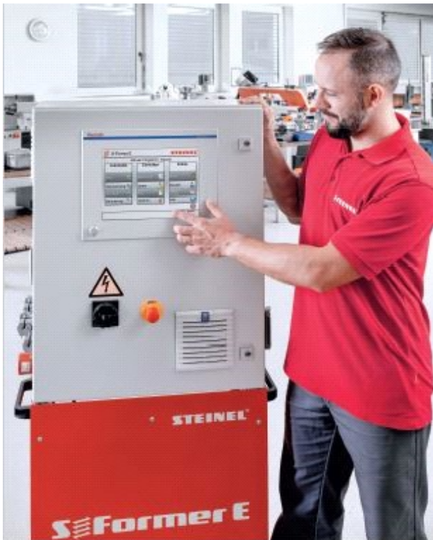
User-friendly: The control unit of the S-Former E with 12" touch display
