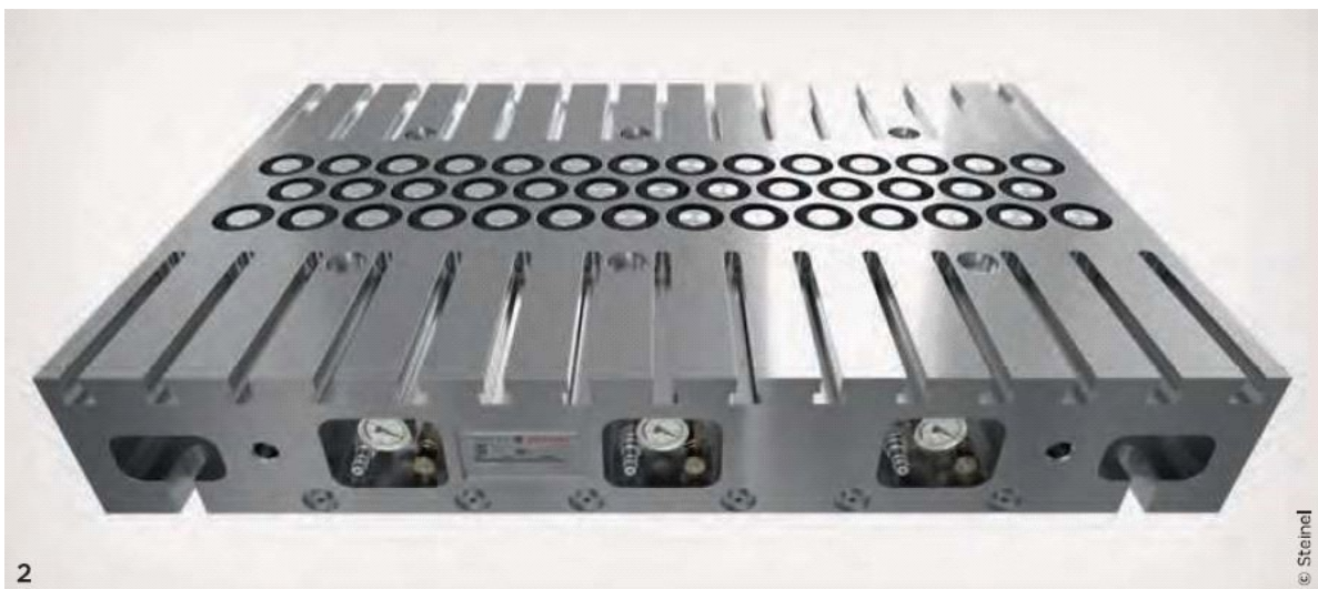
2 Manifold plate with three pressure circuits that can be set independently of each other. One, two or three pressure circuits can be filled and the respective filling pressure can be adapted to the strip stock that has to be machined.
